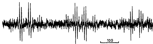
Fig. 6. The EPR spectrum of the radical ion generated from quinoxaline in trifluoroacetic acid with thallium(III) trifluoroacetate as oxidizing agent at 261 K.
